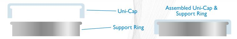
The **Uni-Cap** dust cap seals are designed and developed undersized. The basis of this is so that the **Uni-Cap** is stretched over the support ring to achieve an optimum seal.
